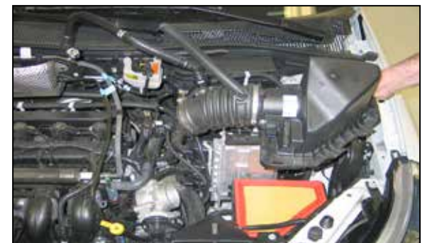
6. Remove factory intake hose and airbox lid from the vehicle.
