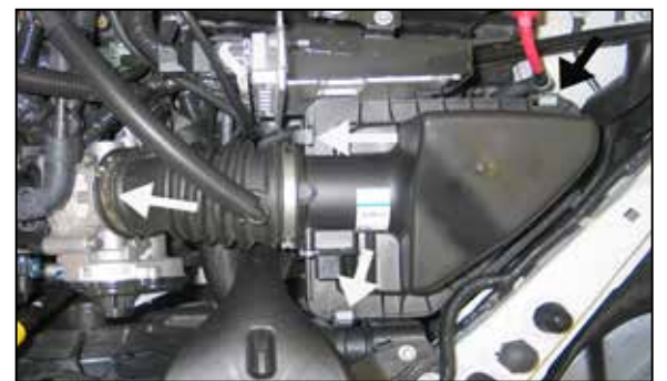
5. Release the three retaining clips securing the airbox lid and loosen the hose clamp at the throttle body.
