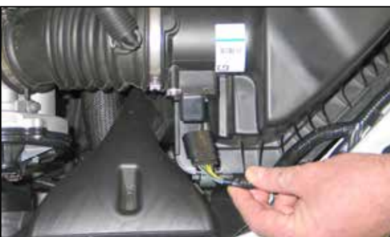
2. Disconnect the mass air sensor electrical connection.
