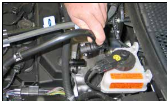
3. Release the locking tab and then disconnect the crankcase vent line from the rear of cam cover as shown.
