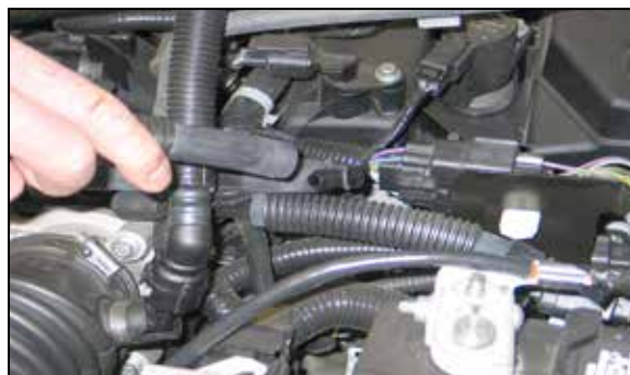
4. Remove EVAP hose from the EVAP valve as shown.
